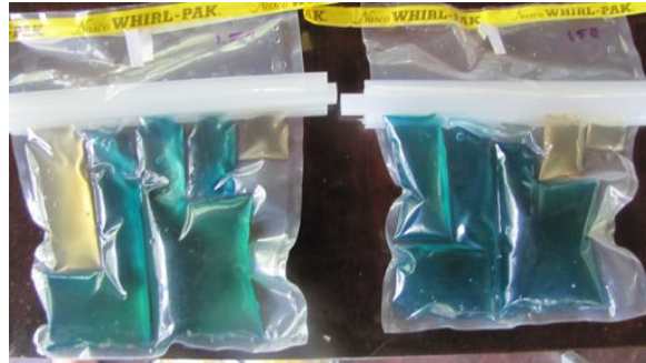
Figure 3 Photograph of the compartment bag test in use in the field.
